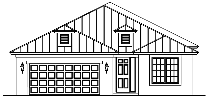
FRONT ELEVATION - TRADITIONAL W/ METAL ROOF
